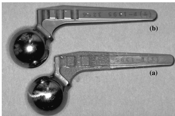
Figure 1 The two types of implants: (a) Metaphyseal sandwich coated implant, (b) Uncoated implant.
